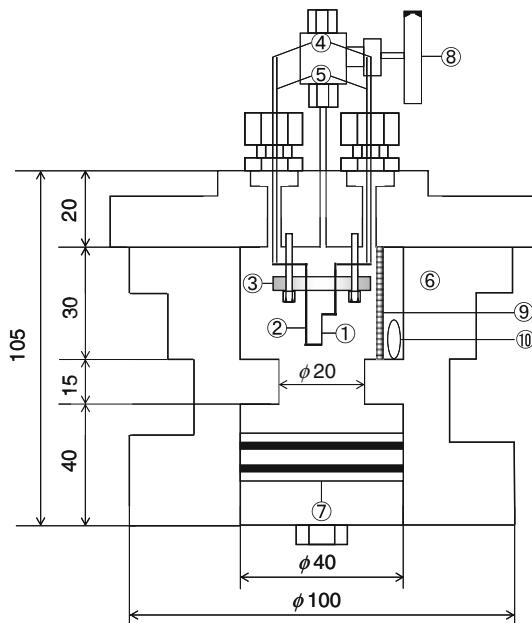
cell,  $\text{CO}_2$  was introduced into the cell from a valve. The amount of  $\text{CO}_2$  charged in the cell was determined by weighing the cell with the use of an electrical balance. In order to obtain homogeneous conditions, the mixture was stirred with a magnetic bar at ambient temperature and 10.0 MPa for 1 day.
