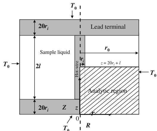
The values of  $a$  and  $b$  were determined by least squares from a plot of  $\ln t$  versus  $\Delta T$ . When the probe was heated, the wire temperature increased but the lead terminal temperature remained at the initial temperature. The correction in the probe temperature rise is similar to that of Fujii et al. [5]. The temperature of the probe increased from 1 K to 3 K after 1 s.
